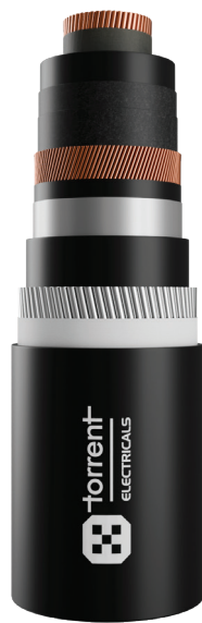
COPPER WIRE SCREEN POLY-AL-POLY SHEATH 132 kV
